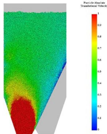
**Figure 9** Snapshot of Eccentric Discharge in Silo with Material Build-up (DEM)
