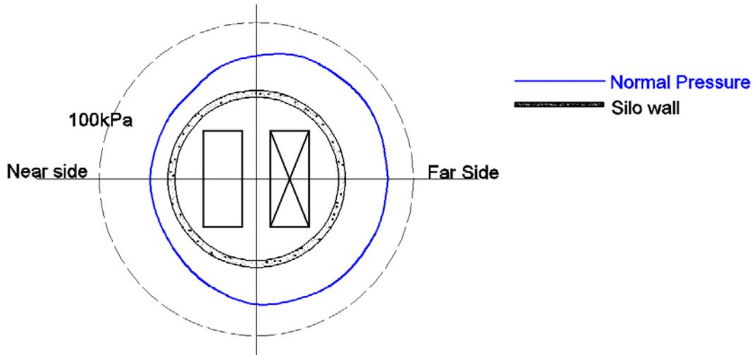
**Figure 6** Numerical Results for Pressure Distribution around Silo Periphery at 1 m above Transition Level
