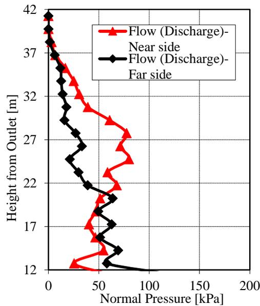
**Figure 5** Numerical Results for Normal Pressure on Cylinder Section of Silo during Eccentric Discharge
