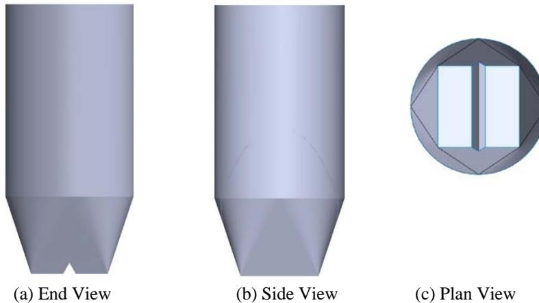
**Figure 1** Configuration of the Simulated Silo
