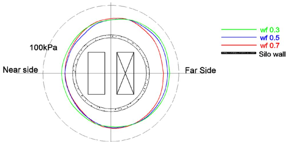
**Figure 8** Wall Friction factor vs. Normal Pressure Distributions around Silo Periphery at 1 m above Transition Level
