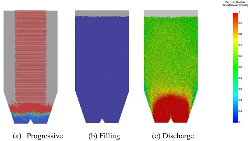
Figure 2 Simulation of Filling and Empty
