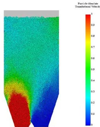
**Figure 4** Snapshot of Material Eccentric Discharge (DEM)
