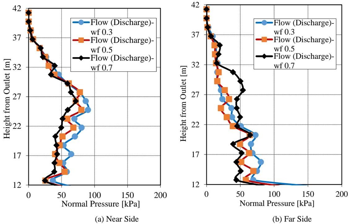
**Figure 7** Effect of Wall Friction coefficient on Normal Pressure on Cylindrical Section - Eccentric Discharge
