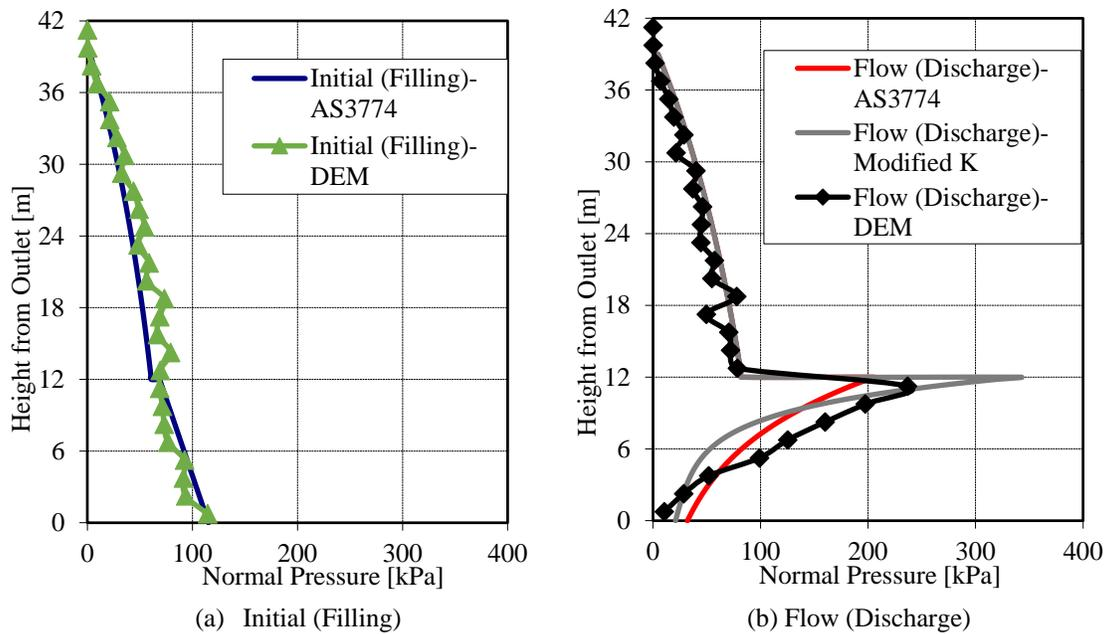
Figure 3 Normal Loads during Filling and Discharge
