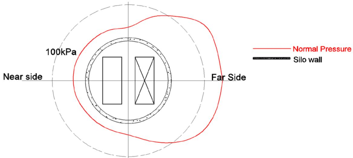
**Figure 10** Pressure Distribution around Silo Periphery at 1 m above Transition Level (Material Build-up in Silo)
